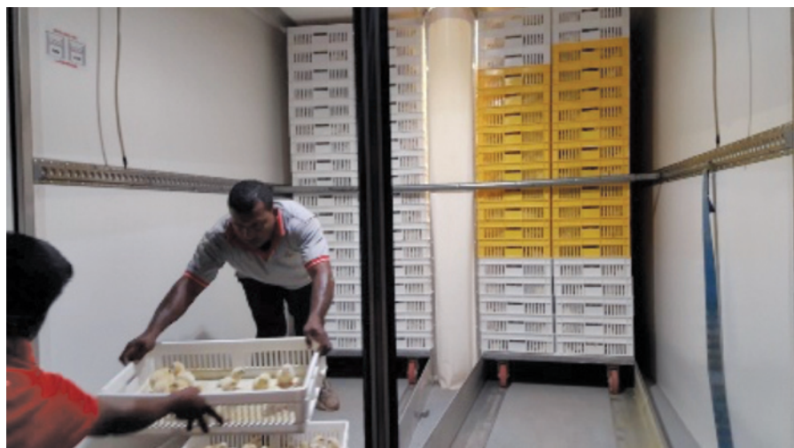
External chick delivery with the Heering V-shape truck. The white curtain in the V-shape supports the airflow in the partial load.
